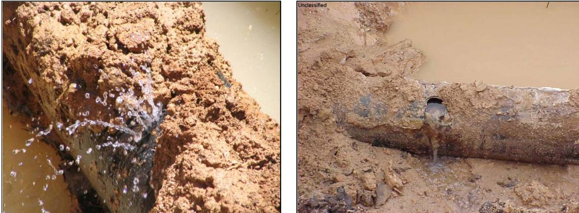
Figure D-16. Fire Protection Lead-In Piping Corrosion.
