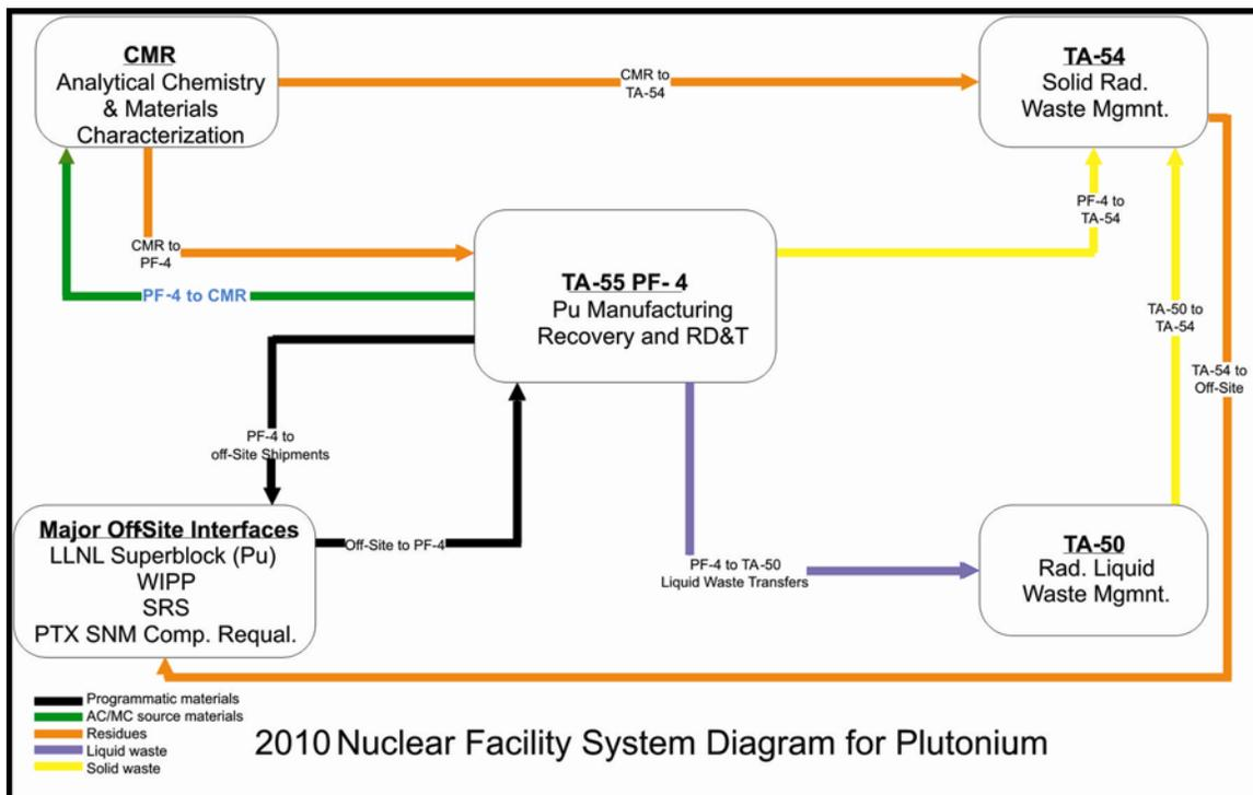
Figure D-7. Key LANL Plutonium Facilities in 2010.
