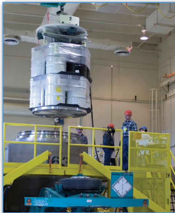
Packaged drums of TRU waste are lowered into a shipping container for transportation to WIPP.
