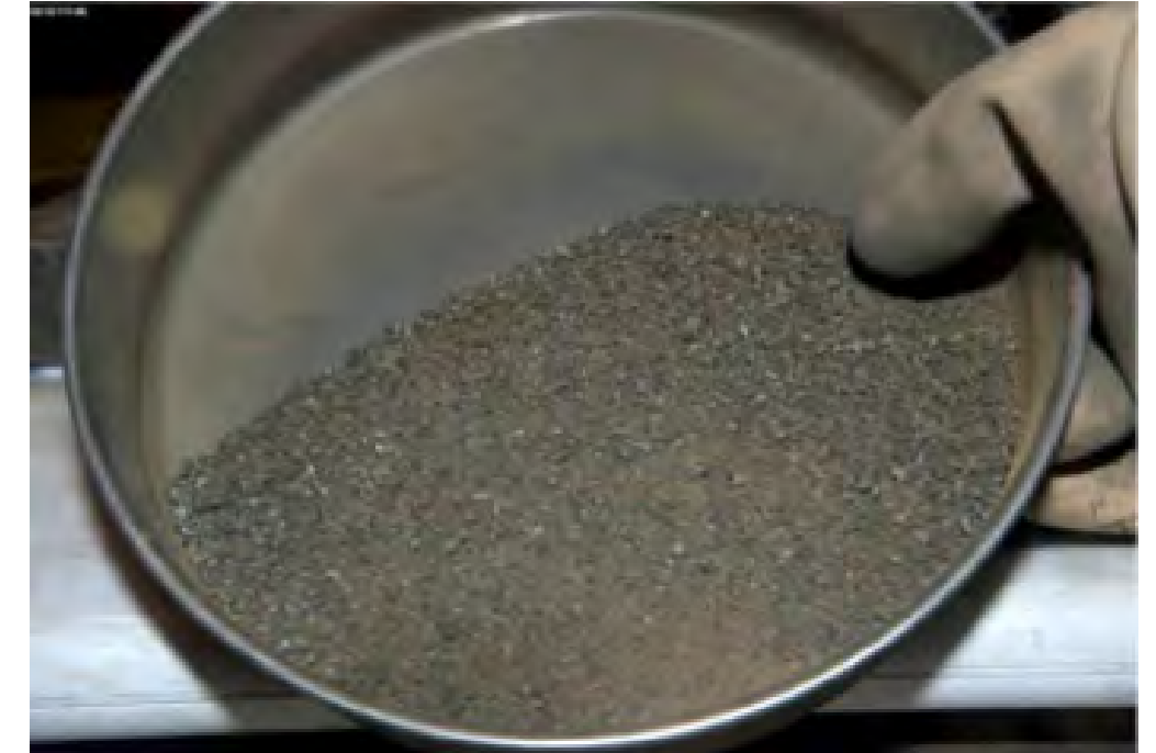
Plutonium oxide produced at the Plutonium Facility at Los Alamos National Laboratory.
