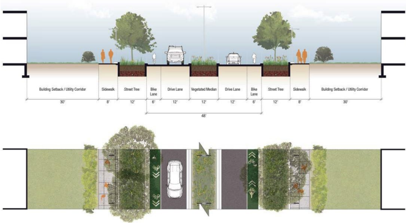
Figure 6-B: Road section diagram—campus arterial road.
