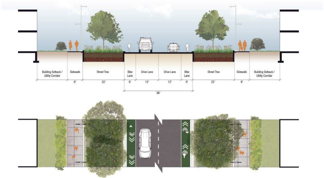
Figure 6-C: Road section diagram—LANL engineering standard.
