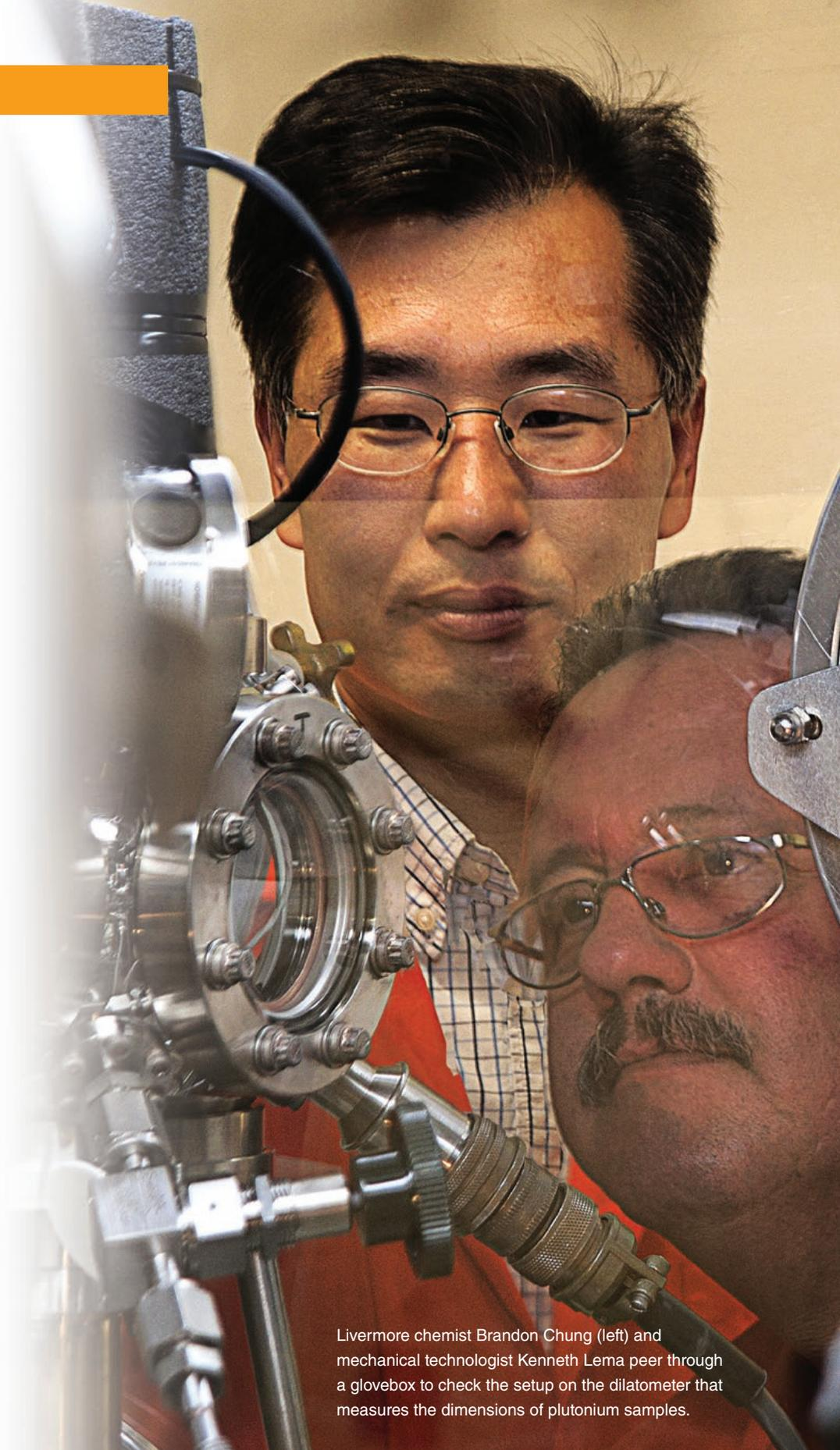
Livermore chemist Brandon Chung (left) and mechanical technologist Kenneth Lema peer through a glovebox to check the setup on the dilatometer that measures the dimensions of plutonium samples.
