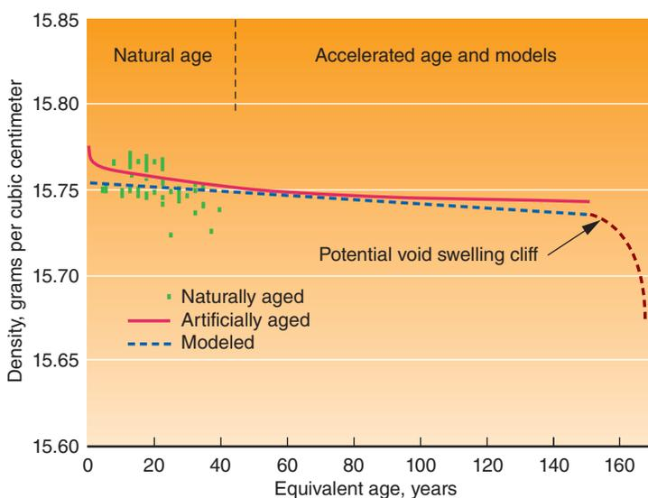
Small changes in density in naturally and artificially aged samples indicate that pits made from a plutonium-239 alloy will retain their size, shape, and strength despite increasing damage from self-irradiation. Results from long-term dilatometry experiments have increased confidence that the pits will function as designed up to 150 years after they are manufactured.
