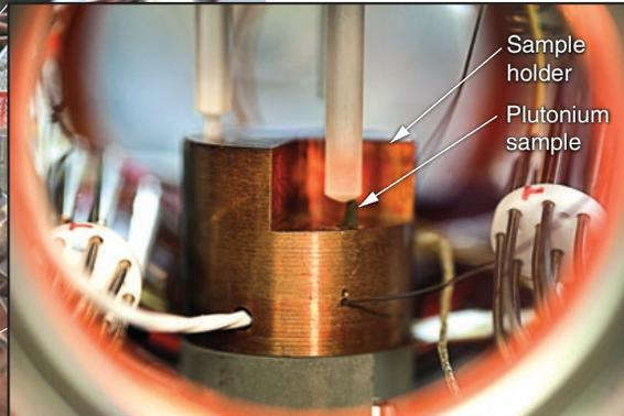
Samples of naturally and artificially aged plutonium, each only 2 or 3 centimeters long, are measured in dilatometry experiments to check for changes in a sample's volume over time.
