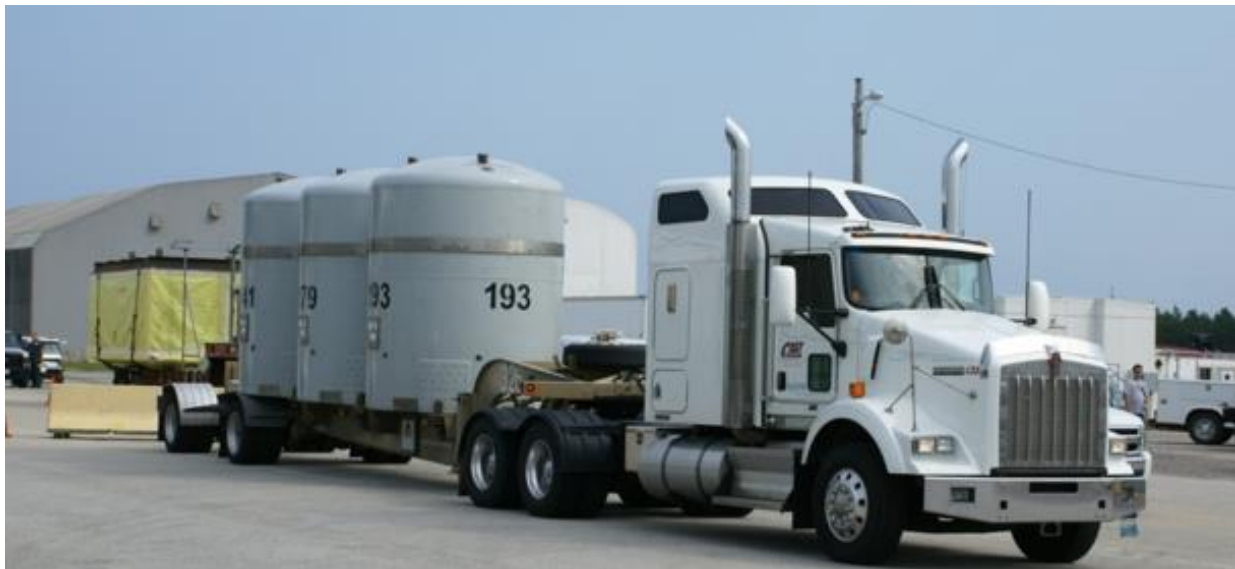
Figure S-16. TRUPACT-II Transporter Used for Shipping CH-TRU Waste to the WIPP Facility
