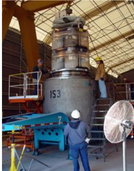
Figure S-15. Drums Loaded into a TRUPACT-II for Transport
