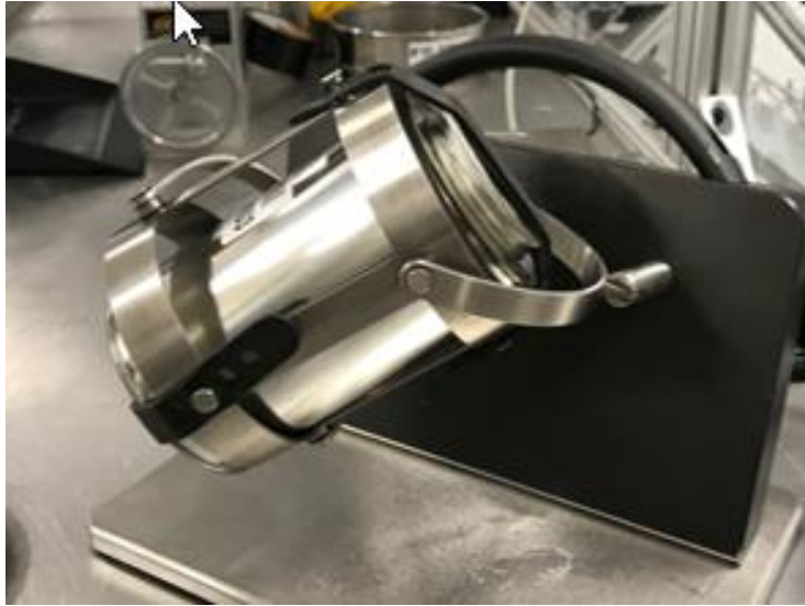
Figure S-12. Blending of Plutonium Oxide and Adulterant in a Blend Can
