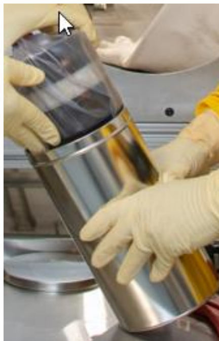
Figure S-13. Diluted Plutonium Oxide CH-TRU Waste Packaged in a Can/Bag/Can
