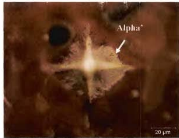
Figure 6. The stress of the Vickers hardness indentation has transformed the delta (dark phase) to alpha' (light phase).
