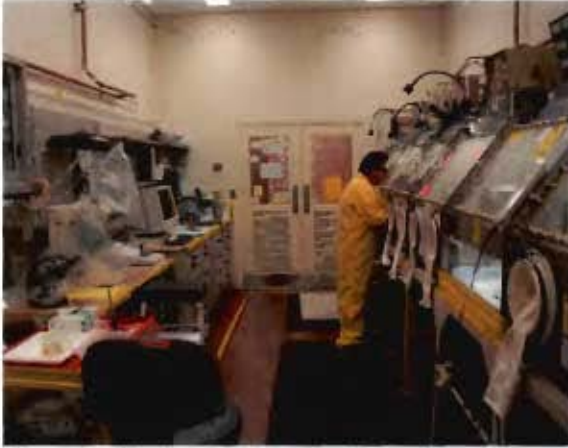
Figure 1. This is a photograph of glove boxes in the R&D plutonium metallography laboratory.
