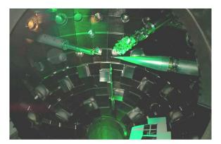
*Figure D-4. Interior of NIF chamber.*
