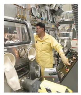
Figure D-10. A machinist operates a precision lathe inside a glovebox.
