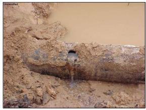
Figure D–16. Fire Protection Lead-In Piping Corrosion.
