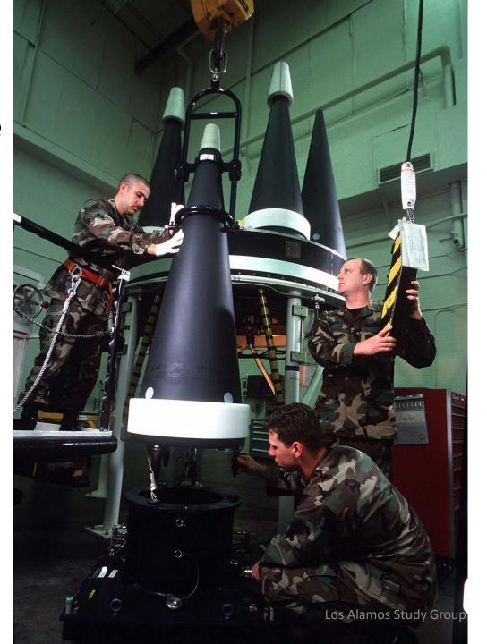
W87-0 in Mark 21 reentry vehicles (RVs), shown here in (retired) MX missile configuration. Circular error probable (CEP) is classified but say ~100 m, with "smart" fuzing. Yield is 300 kilotons (kt), with a 475 kt variant optional. It is pits of this type which LANL is tasked to make.
