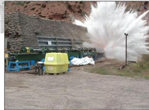
Large bore powder gun – measure differences in performance of weapon materials of interest
