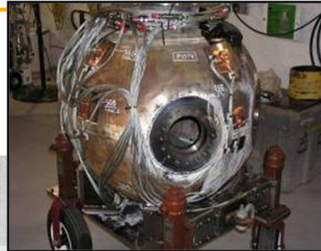
Barolo experiment Vessel - measure the effects of a shock on a plutonium surface.
