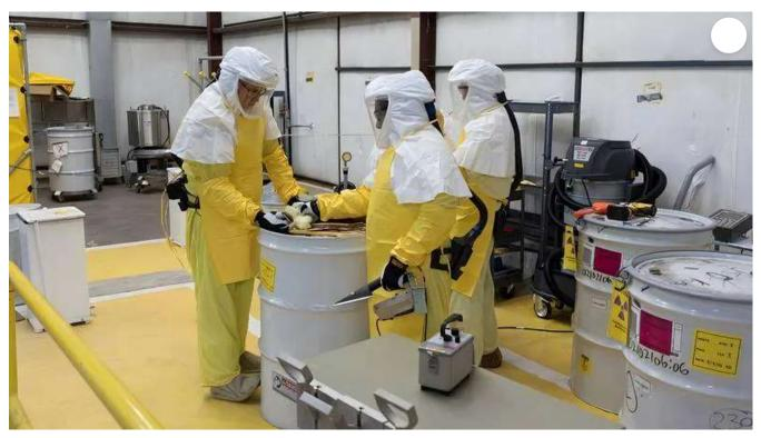
Workers with EM Los Alamos Field Office cleanup contractor Newport News Nuclear BWXT Los Alamos use a new processing line to process and repackage drums of low-level nuclear waste for disposal offsite at Los Alamos National Laboratory's Technical Area 54. (Courtesy Department of Energy)
